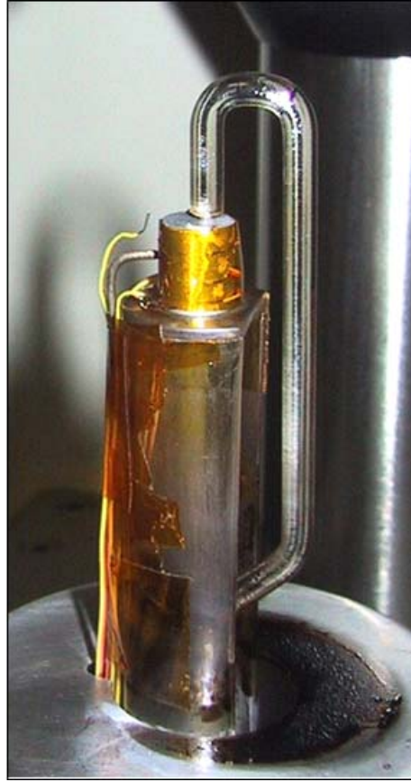
Figure 6(a): An aluminum sample with TCs taped to the side was used to measure the temperature gradient within the sample.
