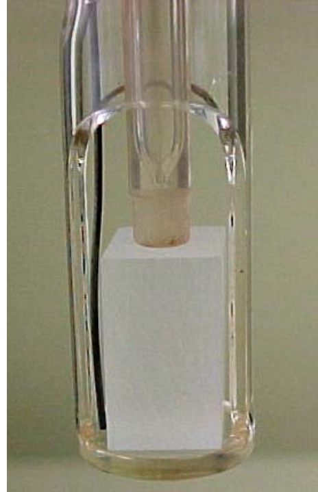
Figure 1 Arrangement of the sample on the TMA stage under the probe and the position of the thermocouple.
